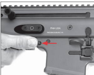
Push in on the takedown pin from the left side.
