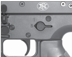
"Safety" shown in the on safe position.
