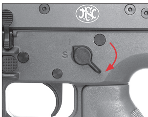
"Safety" shown in the off safe position.
