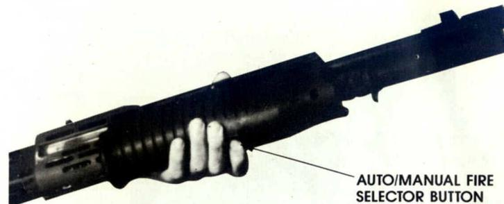
The auto/manual fire selector button is on the bottom of the forend. It can be pressed with a finger of your non-firing hand without changing your normal grip on the shotgun.
